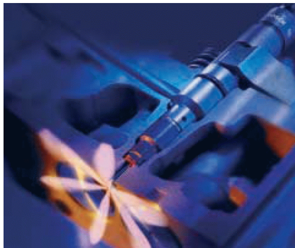
Figure 3: Future fuel injector for diesel engine with nanometer thin diamond like coatings 2
